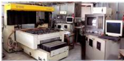
MITSUBISHI LASER 1212HC 1992 1600 WATTS CO2 LASER 3016F2 Includes Chiller & Cooling Tower
